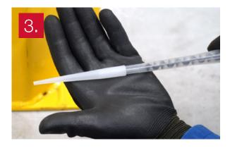
3. Stick mixer reducer tip on static mixer nozzle. Adhesive tape can be used if necessary.
