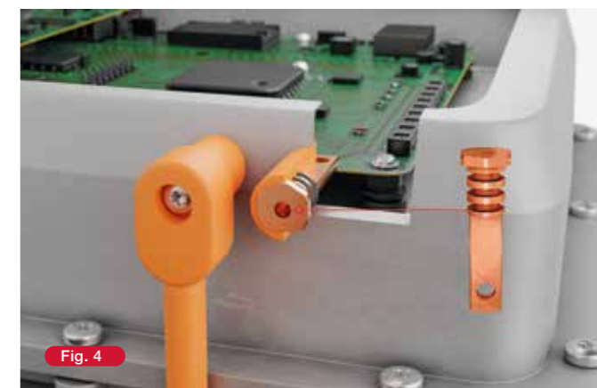
Fig. 4 EJOFORM® Copper Contacts with High Electrical Conductivity
