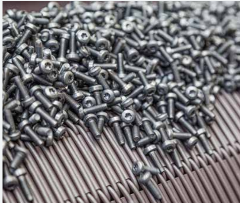
Screws are cooled to below 50 degrees Celsius at the end of the tempering furnace, the heat of the cooling flow is used to preheat the screws before they reach the tempering furnace.
