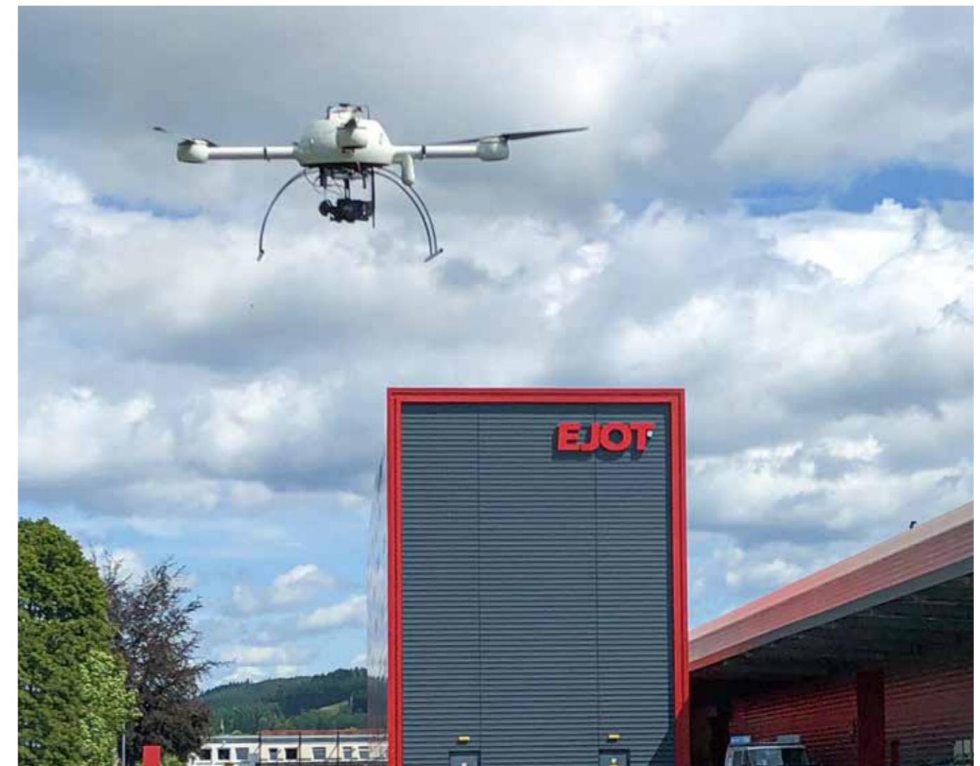
The measurement of the existing building is carried out with a drone and is automatically transferred into a 3D model through the development of a digital construction in the software.
