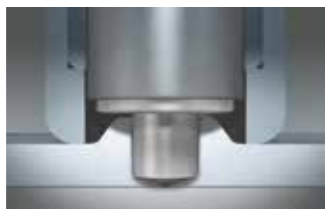
Phase 2: Surface cleaning and activation
