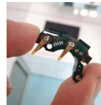
Micro screws in the sound processor
