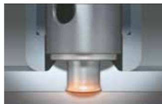
Phase 3: Plastification of friction element and base sheet
