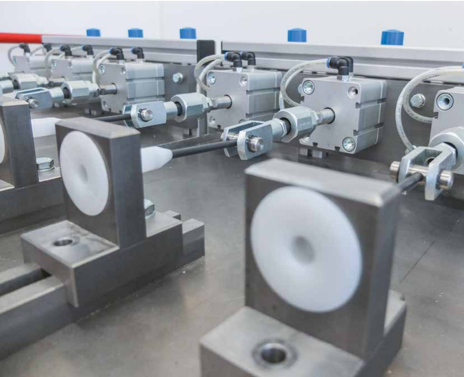
Permanent load tests in the laboratory monitor the product quality
