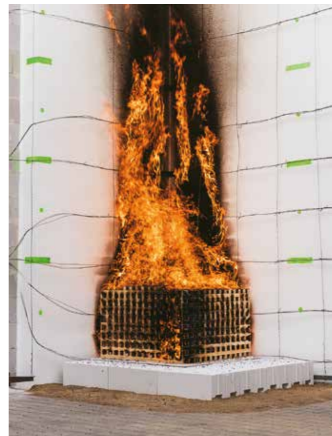
MPA Dresden GmbH facade test stand (left inner view with test stand) with a height of up to four full floors.
