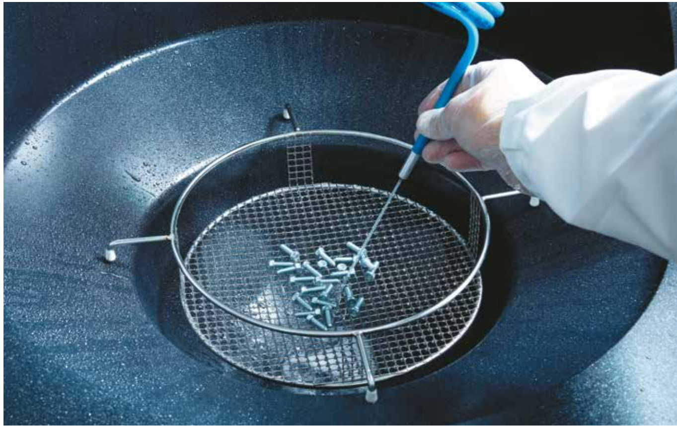
Extraction process of a cleanliness test according to VDA 19 / ISO16232
